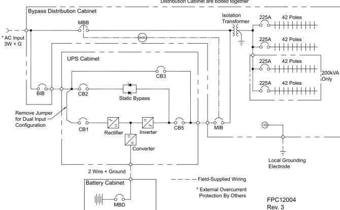
UPS AC input and AC output cables are factory-supplied when UPS and Bypass Distribution Cabinet are bolted together
